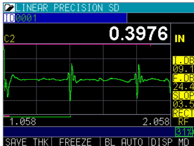
Class 1 with cursor on first backwall echo
