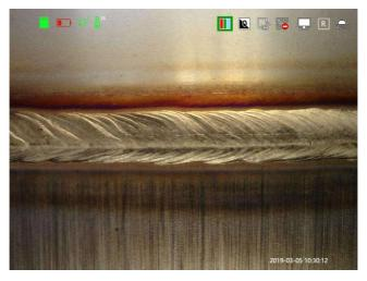
Temperature indicator is on the upper left of the screen. When the testing temperature is 20°C~64°C, it indicates in green color. Orange alarm when the probe temperature is 65°C~79°C; red alarm when above 80°C. For the protection of the probe and camera, the monitor will shut off automatically.
