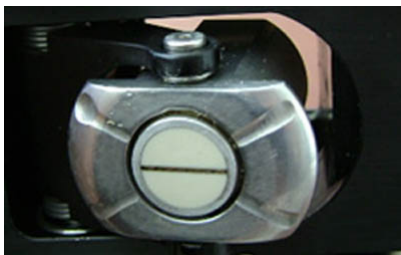
Detail of spring loaded transducer
