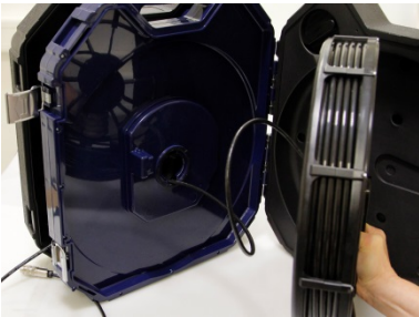
Fig. 66: Removing the viper with the connection cable from the case.
