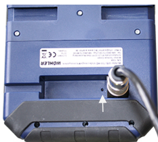
Fig. 60: Reset hole indicated by an arrow
