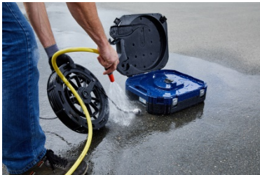
Fig. 68: Cleaning the viper and the rod
